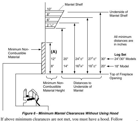
If above minimum clearances are not met, you must have a hood. Follow minimum clearances shown in Figure 7 when using hood.
